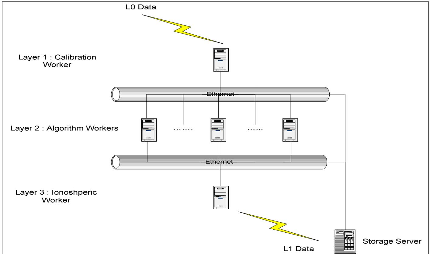
**Figure 7: Proposed Architecture for the L1 processor**
