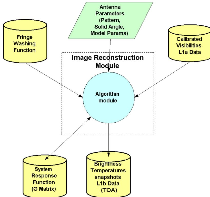
**Figure 11: Image Reconstruction Module**
