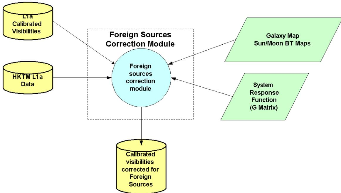
**Figure 10: Foreign Sources Correction Module**
