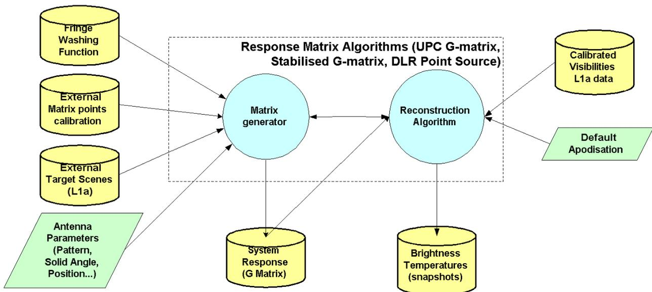
Figure 14: Response Matrix Algorithm Module
