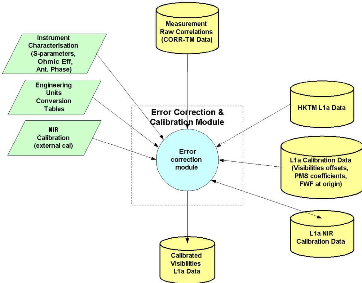
**Figure 9: Calibration and Error Correction Module (Measurement Data Processing)**
