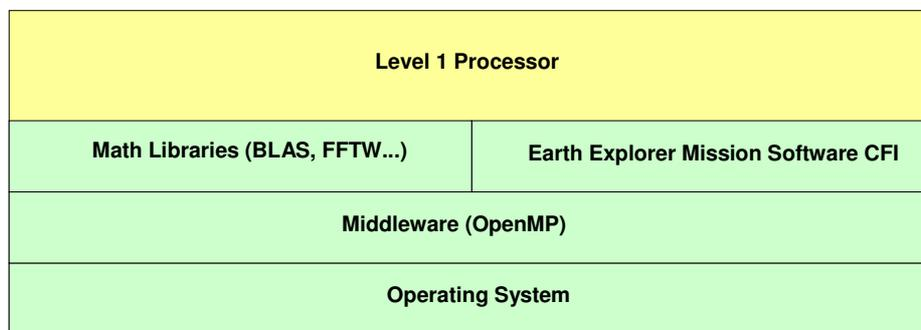
*Figure 6: Level 1 Processor Software Layers Example*
