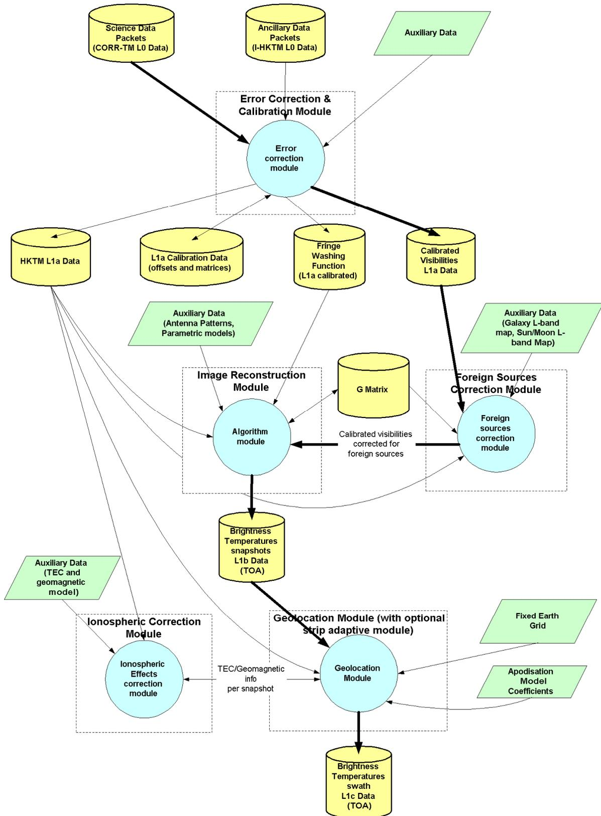
**Figure 3: Processing Data Flow Diagram**
