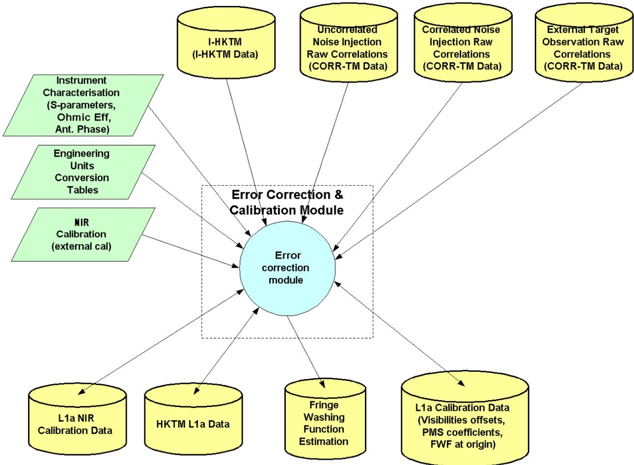
**Figure 8: Calibration and Error Correction Module (Calibration Data Processing)**
