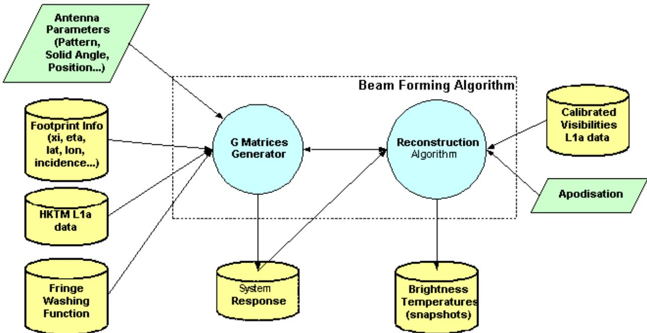
**Figure 16: Beam Forming Algorithm Module**
