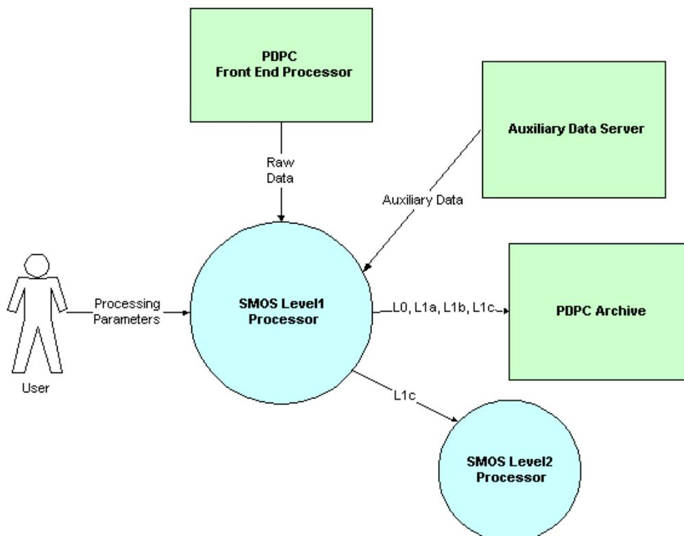
**Figure 2: SMOS L1 Processor Context Diagram**
