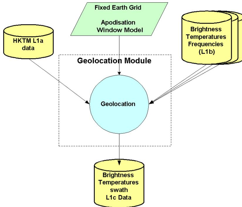
**Figure 12: Geolocation Module**
